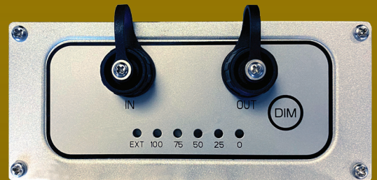
Onboard Dimmer & External Dimming connections
